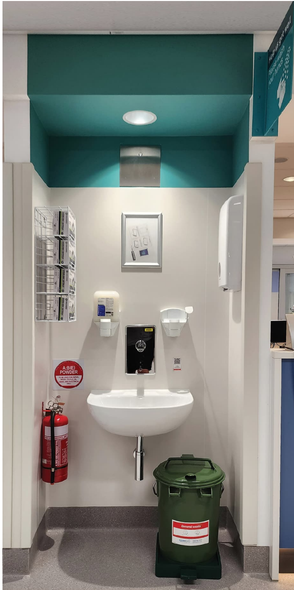
Figure 04 - Purposeful graphic devices can be used to mark handwash stations to drive a culture of good hygiene practices. Photo credit: Jacobs.
